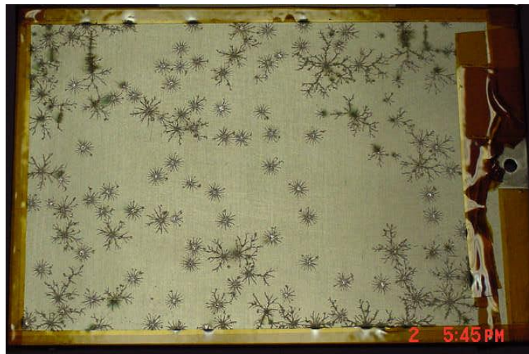
Figure C.9 — Anodized aluminum plate after repeated arcing (Schneider et al., 2002, p. 2)
