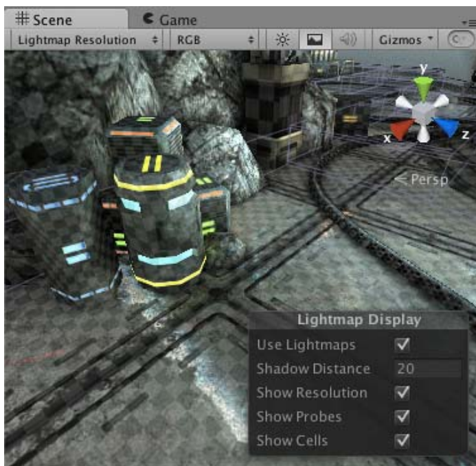
Lightmap Resolution scene view mode visualising how the lightmap texels are spent (each square is one texel).
