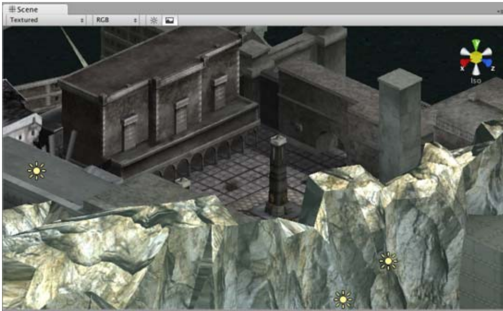
Orthographic camera. Objects do not get smaller with distance here!
