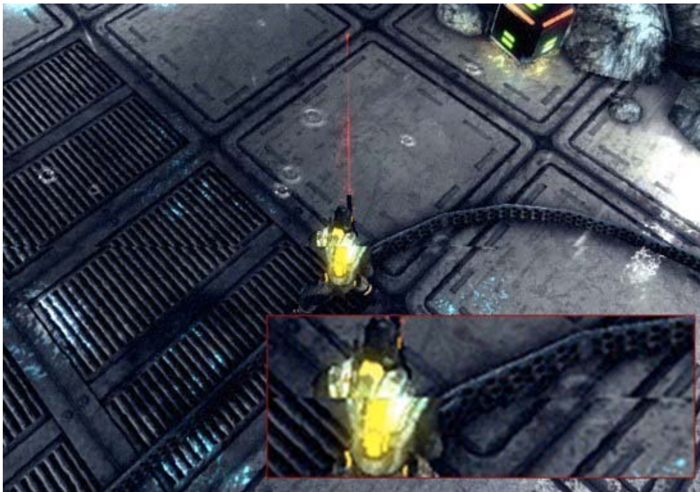
Simulated example of tearing. The shift in the picture is clearly visible in the magnified portion.
