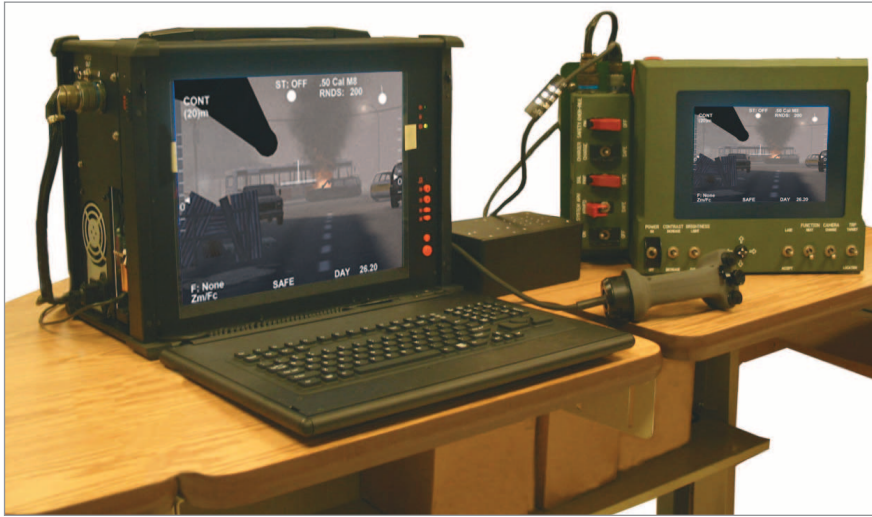
Figure 1. Common remotely operated weapon station basic skills trainer. The BST integrates fielded hardware with the AA gaming engine software.
