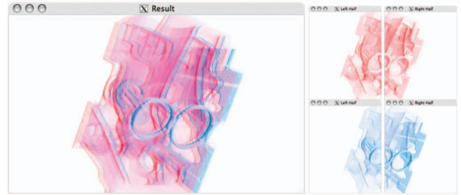
Fig. 21. Four-to-one stereo/sort-first parallel volume rendering.
