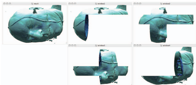
Fig. 18. Demonstration of direct-send image compositing in combination with \alpha -blended volume rendering. Each node renders one volume slab as well as composites one horizontal image stripe for final assembly, which is displayed in the upper left window.
