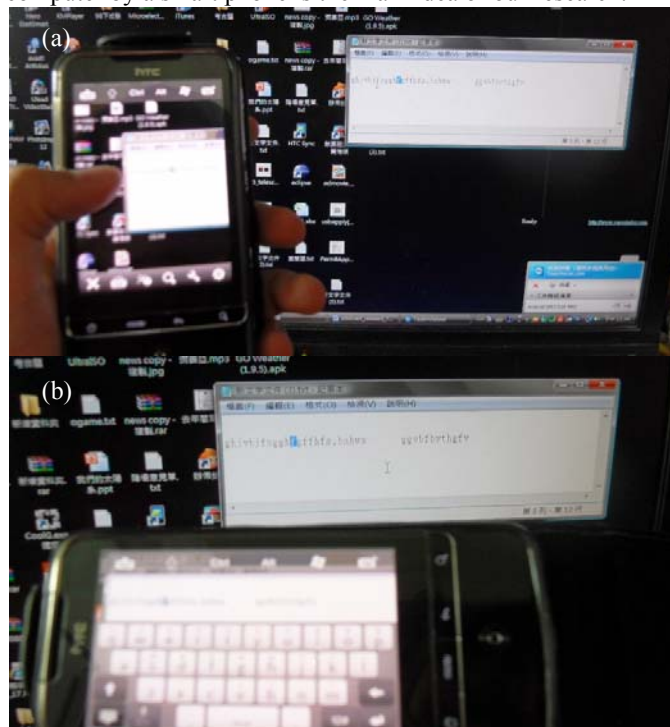
Fig. 3. The schematic of the TeamViewer. (a) Slide finger on the smart phone screen can control the mouse cursor on computer screen. (b) Using the virtual keyboard built-in the smart phone to key words can replace the function of physical keyboards.
