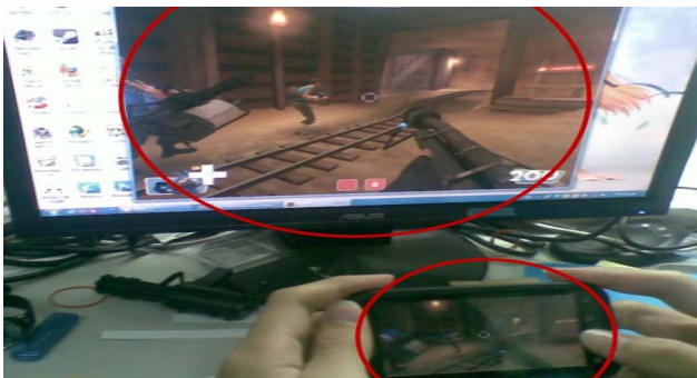
Fig. 2. The schematic of the system. The PC screen displays an executing PC-based FPS game. The smart phone is the controller of the PC game in this system.
