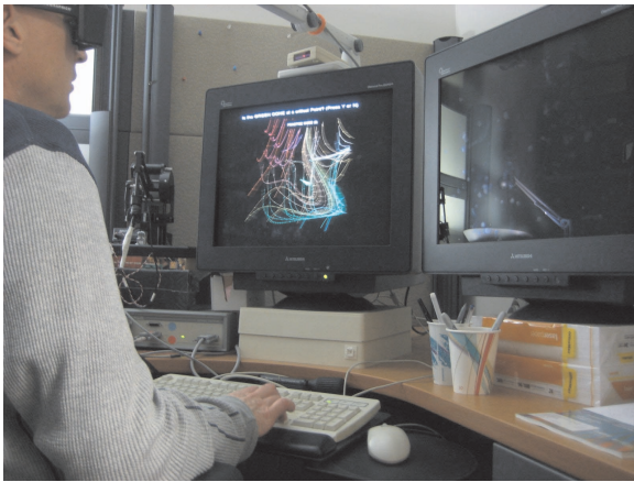
Fig. 1. A participant views 3D vector field visualizations at a stereo monitor, wearing active stereo shutter glasses for both stereoscopic and monoscopic visualizations. The keyboard is used both to rotate the dataset and to specify answers and confidence levels.
