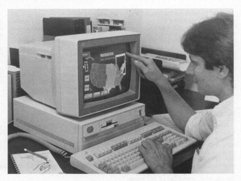
MicroTouch's line of touch-screen products for the IBM PS/2 consists of touch monitors based on IBM and Magnavox monitors, touch-screen kits, and a software development system.
