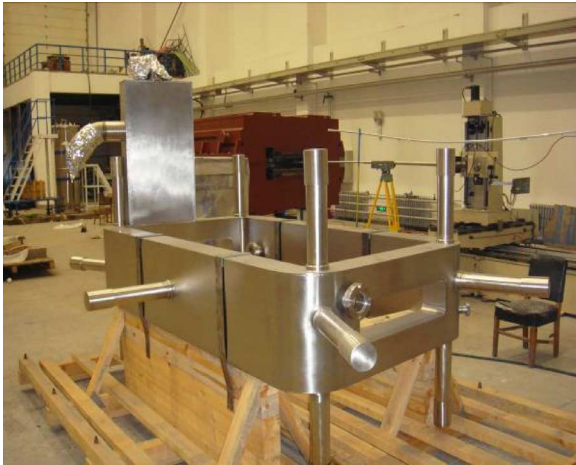
Fig. 17. Configuration of dipole magnet for GSI CR ring.
