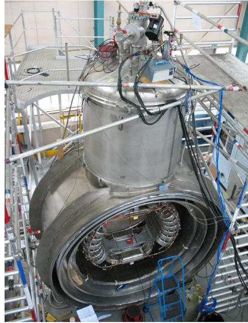
Fig. 10. Test cryostat for Alpha magnetic spectrometer-02 (fabricated:2006).
