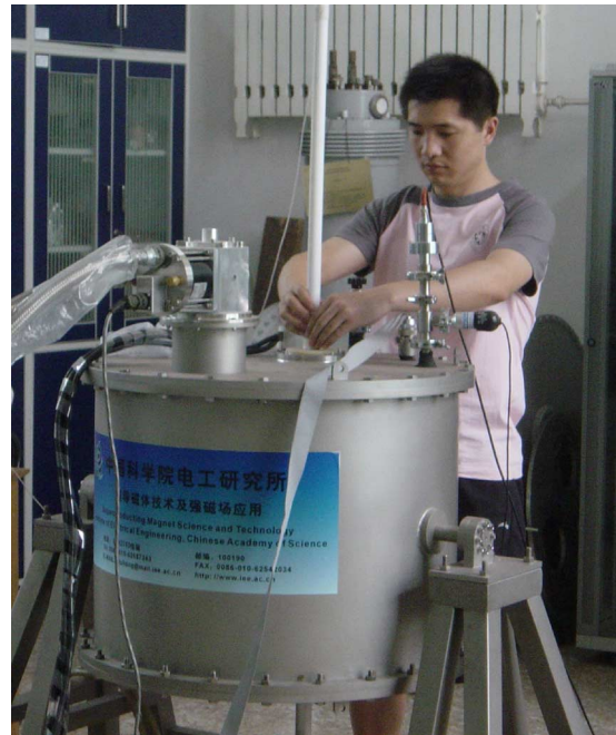
Fig. 2. High magnetic field conduction-cooled superconducting magnet with warm bore size of 100 mm and center field of 10 T (fabricated: 2009).
