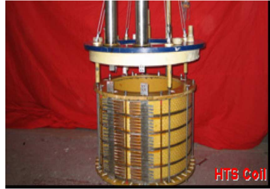
Fig. 20. HTS coil for 630 kVA/10.5 kV/0.4 kV three-phase.
