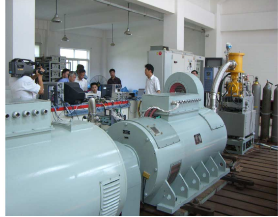
Fig. 23. Configuration of 30 kW motor with HTSC cooled by liquid N_2 .
