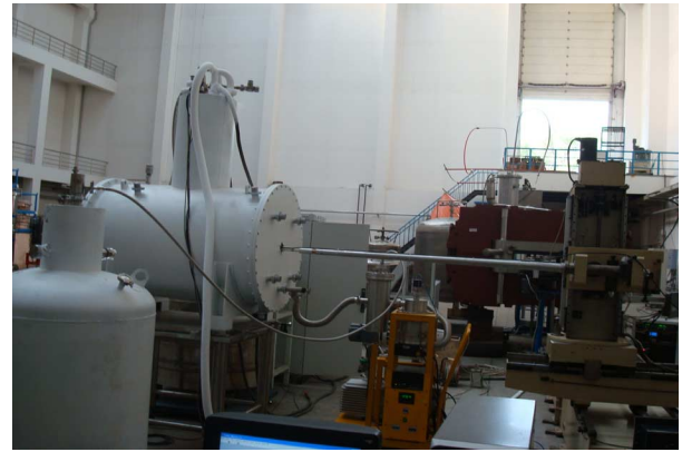
Fig. 11. 3 T solenoid, cryostat and measurement system.
