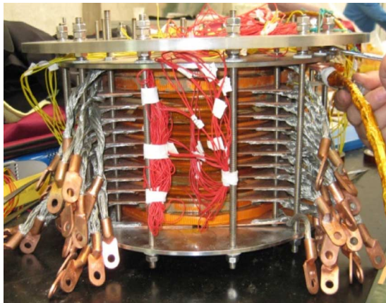
Fig. 22. HTS coil for SMES fabricated in CEPRI Race-track-shaped superconducting coils.
