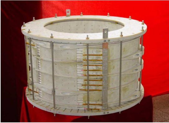
Fig. 18. The 10.5 kV/1.5 kA three-phase SFCL by IEECAS.
