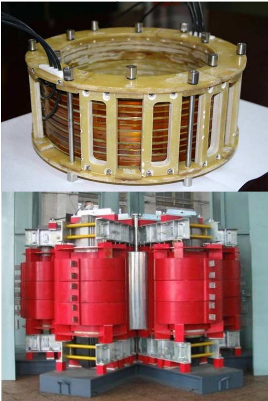
Fig. 19. HTS coils used in 35 KVA SCFL in InoST Power.
