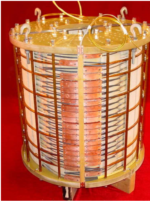
Fig. 21. HTS coil for 1 MJ SMES fabricated in IEECAS.
