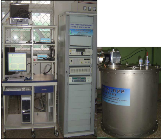
Fig. 4. The test bed for the HTS tape and LTS wire (fabricated:2007).
