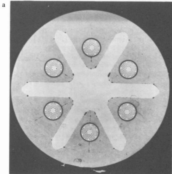
**Figure 5a** Photograph of cross section of new conductor, constructed as shown in **b**. Solder bonds are visible due to etching. Full scale conductor for 5500 MW h is 13.5 cm diam. or 400 strands of 0.6 cm (after WSESP 1977)
