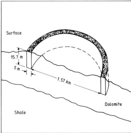
**Figure 3** Three dimensional view of low aspect ratio 5500 MW h solenoid in a surface trench in bedrock
