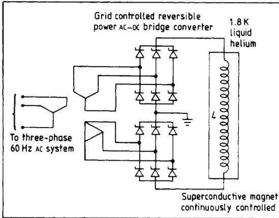
**Figure 1** Circuit diagram of AC-DC power converter and inductor (after Boom, Peterson et al 1974)
