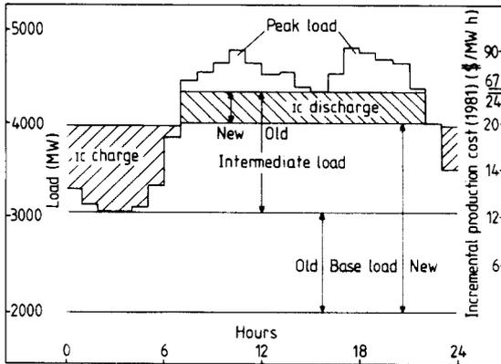
**Figure 2** Load curve for January 1995 produced by WEPCO planning department: hatched areas show possibilities of IC charging and discharging
