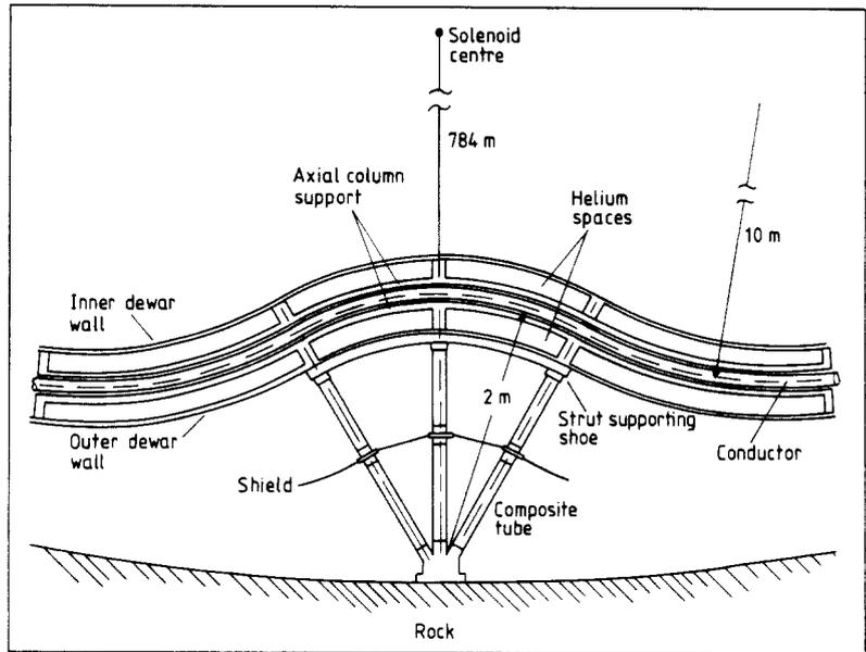
circular pattern so that forces in each tunnel are directed radially outward without shear on a rock face. Here shear is equivalent to the axial load in the low aspect ratio coil. Without shear forces the required axial structure is only 3.2% of the minimum virial theorem mass, mostly in the end two 'field adjustment' tunnels. More information is given in the paper referred to.
