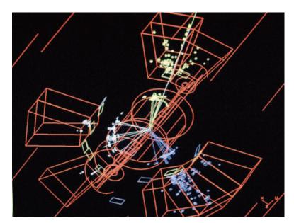
Fig. 1. A photograph from the L3 collaboration, showing three jets emerging from electron–positron annihilation at high energy. These jets are the materialization of a quark, antiquark, and gluon. (Reprinted with permission of the L3 Collaboration.)
