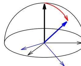
**Geodesic Reference Frame** is the frame found by tilting North Pole of "canonical frame" along a great circle until it points in desired direction (**tangent for curves**, **normal for surfaces**).
