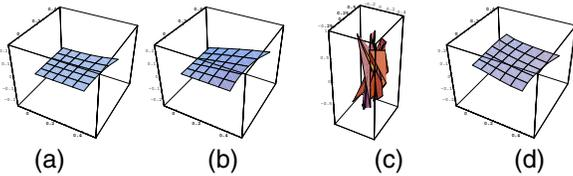
Quaternion frames for (a) Geodesic Ref. (b) One edge Parallel Transport. (c) Random. (d) Minimal area result.
