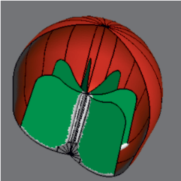
Figure 9: Evolver/Geomview display of spacecraft fuel tank; the fuel surface tension computed with the Evolver is the only force available to guide fuel to the intake valve in low gravity. (K. Brakke, Susquehanna University.)
