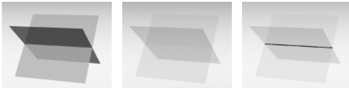
Figure 3. Two intersecting polygons are slightly transparent (left) and very transparent (middle and right). Transparency makes the intersection hard to see, hence the need for highlighting the intersection.
