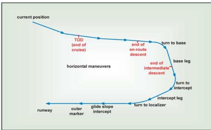
The basis for the trajectory prediction: horizontal maneuvers, altitude and speed profile (compare: "The way OSYRIS Trajectory Predictor works") shown for a trajectory that starts at the current position of a flight in cruise phase.
