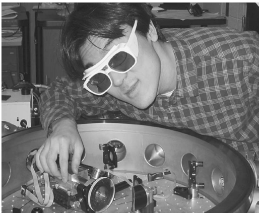
FIG. 29. Progress in laser development. The target chamber of the University of Michigan \lambda^3 laser. This compact laser has a_0^2 \sim 1 with a repetition rate of 1 kHz. This university-size system is the smallest relativistic intensity laser.
