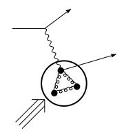
Figure 5.5 Schematic depiction of deep inelastic scattering. An incident lepton radiates a photon which knocks a quark out of a proton. The struck quark is detected indirectly only after hadronisation into observable particles.
