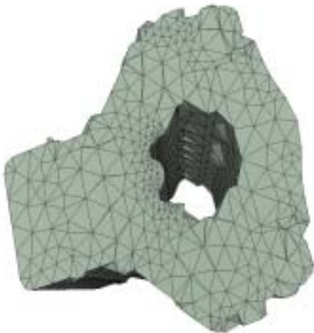
Figure 5: An engine block bounded by a 2-manifold of genus 1.
