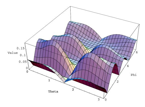
Figure 5: the angular dependence of the total response function of the LIGO interferometer to the magnetic component of a SGW for f = 8000 Hz
