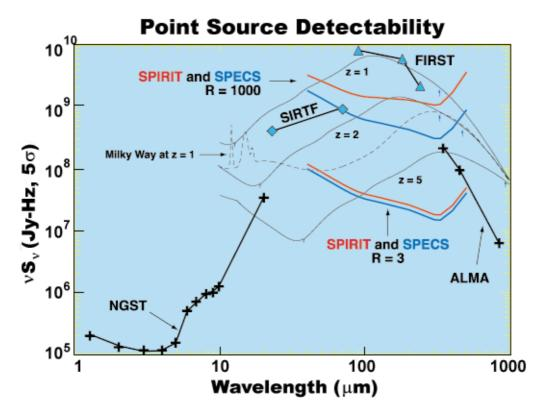
Fig. 1: SPIRIT and SPECS will have sensitivity comparable to that of NGST and ALMA over a spectral range that bridges the gap between them. The FIR/SMM interferometers will be able to measure cooling and diagnostic lines in the spectra of high-z galaxies.
