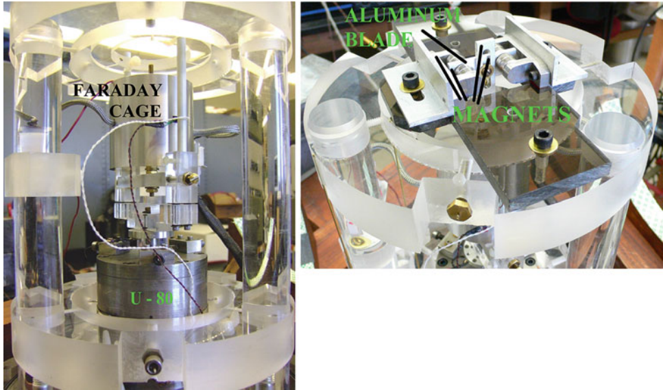
Fig. 5.9 The rod system (also shown in Fig. 4.24) that enables horizontal operation with the U-80 thrust sensor. The upper stabilizing ring and magnetic damper, later additions to this system, are displayed here
