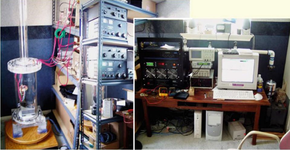
Fig. 4.29 Paul March's home lab. On the left is his vacuum chamber with a test device he built mounted and ready for testing. Some of the power electronics and instrumentation are visible on the right of this panel
