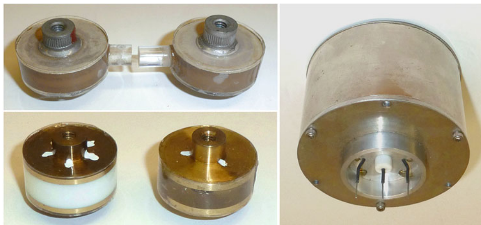
Fig. 4.4 Capacitors ( above ) of the sort used with the system shown in the previous figures, along with dummy capacitors ( below ) used in the system of the previous figures. The capacitor case used (aluminum with mu metal lining) is shown in the bottom right
