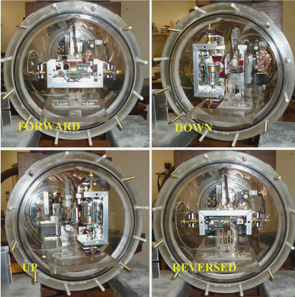
Fig. 5.29 A montage of photos of the device in the Faraday cage (with the top half removed) showing the four orientations for which data was acquired. The forward and reversed, and up and down orientations are differenced. The end plate of the vacuum chamber is removed, and the thrust balance platform slid partly out of the chamber for these photos
