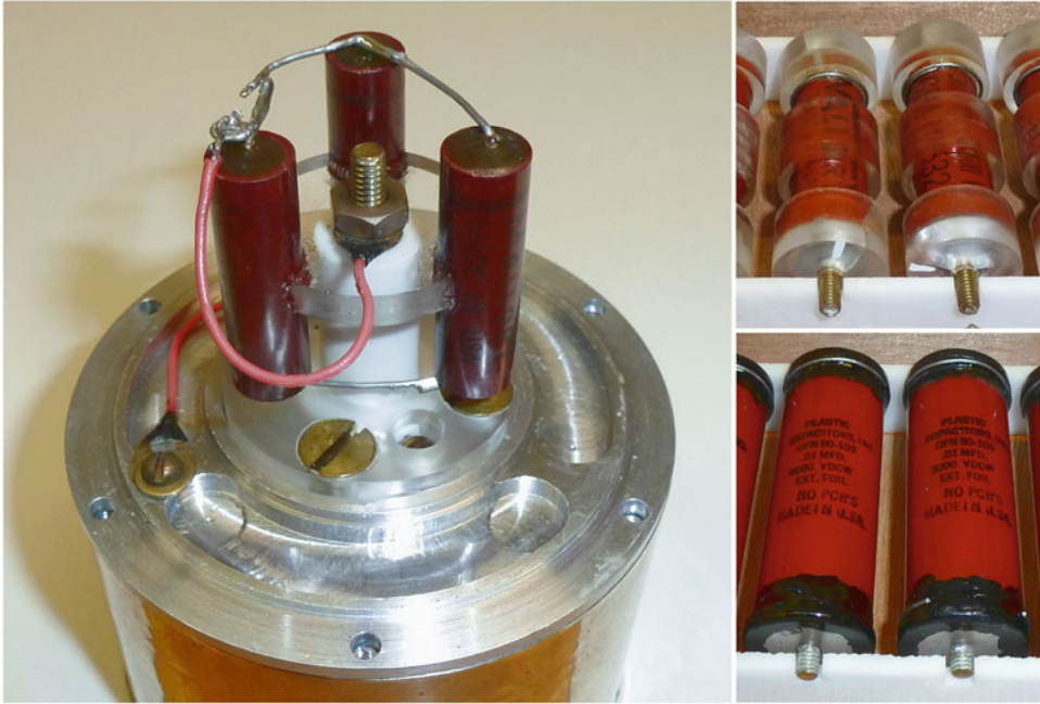
Fig. 4.5 Some of the other high voltage capacitors use in early work on Mach effects. Note that no provision was made to generate “bulk” accelerations in these devices
