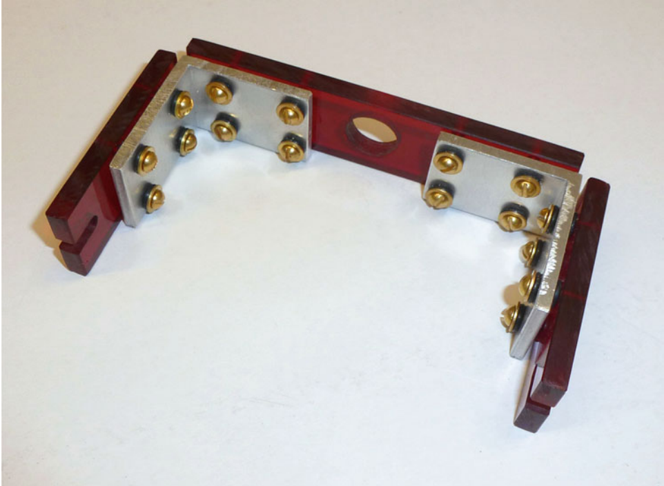
Fig. 5.15 One of the (red) plastic and aluminum fork mounts that replaced the fork mount shown in the picture in Fig. 5.10. The parts of the mount are held together with multiple 4–40 machine screws damped with small Buna-N O – rings and brass washers
