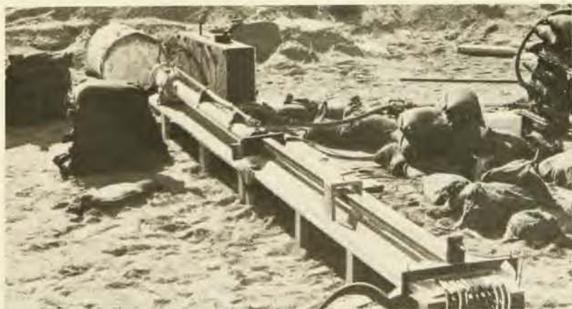
Livermore-Los Alamos rail gun at the Los Alamos firing site. Two 8-foot-long parallel copper strips (foreground) constitute the magnetic-flux-compression generator. Sheet explosive driving the upper strip down generates a megawatt current pulse in the 6-foot-long small-bore rail gun (background). The \frac{1}{2} -inch plastic cube is launched at speeds up to 5.5 km/sec.
