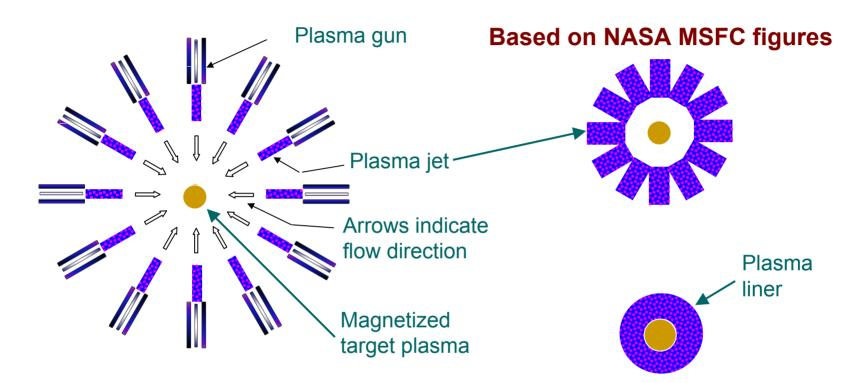
• An approximately spherical distribution of jets is launched towards the compact toroid at the center of a spherical vessel.
