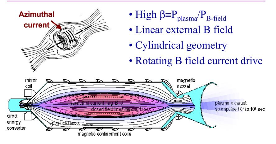
FRC as Power Source and Ion Engine for High Energy Space Missions
