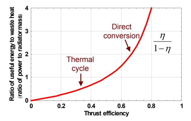
• Doubling efficiency from a thermal cycle's  $\sim 1/3$  to direct conversion's  $\sim 2/3$  gives 4 times better power per unit waste heat.
