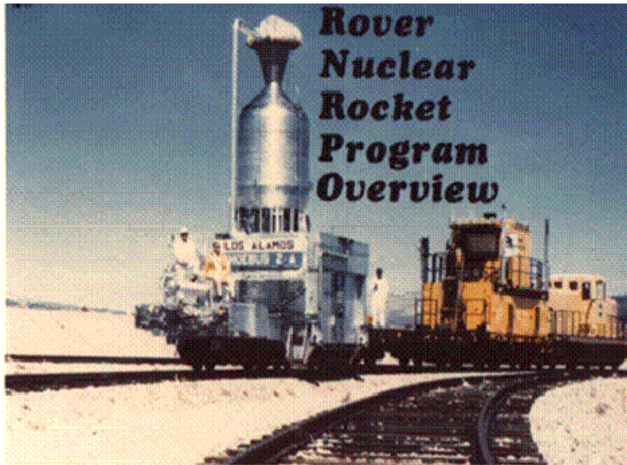
Figure 13 Handling of experimental rocket reactors at the NRDS in Nevada was accomplished by rail. Here the reactor XECF is being moved to the static test site.
