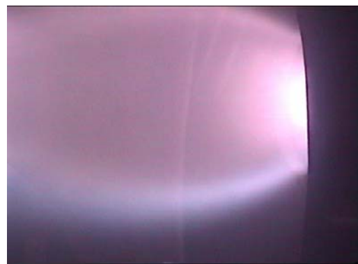
Figure 90 ATILA operating in arcjet mode with superposed induction heating.
