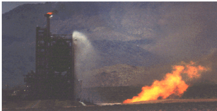
Figure 12 Test of the XE nuclear rocket engine at the Engine Test Stand at the Nevada Test Site. The engine had a thrust of 75,000 pounds and was down firing mounted under a 75,000 gallon tank of liquid hydrogen. The exhaust fired down into a "steam trench." The ETS was constructed only of aluminum to reduce the amount of long lived radioactivity in structural materials induced by the neutrons coming from the engine.
