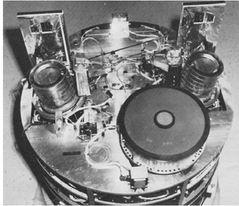
Figure 31 The two Kaufman-type thrusters mounted on the SERT II spacecraft (NASA photo).
