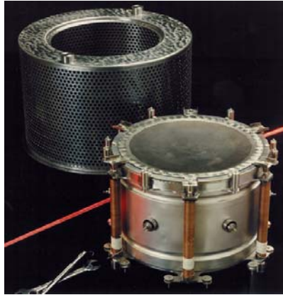
Figure 37 UK-25 engineering model ion thruster with earth screen removed (Culham Laboratory photo).
