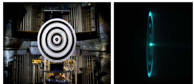
Figure 14. NHT installed at Univ. of Mich. Test facility (left); 30kW hotfire test (right)
