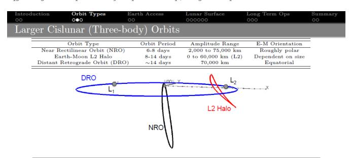
Near-rectilinear halo orbits (NROs) were discovered as a bridge between L1 and L2 halos. NROs are halo orbits with large amplitudes over either the North or South poles that are fixed in the Earth-moon plane.
