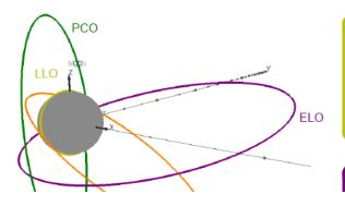
Low Lunar Orbit (LLO): LLO is defined as a circular orbit of an altitude around 100 km. LLOs are favorable for surface access and polar orbit inclinations offer global landing site access.
