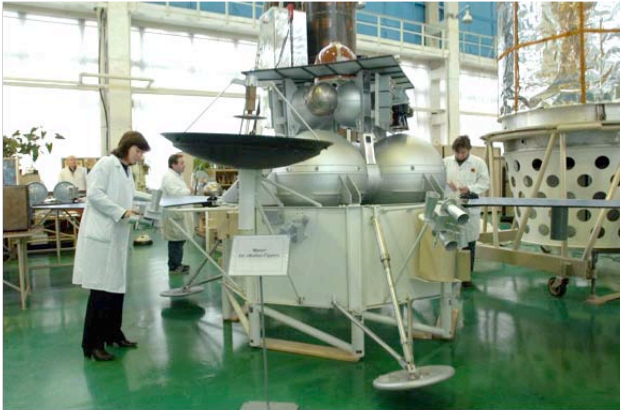
Figure 12: The Phobos-Grunt spacecraft. The dome-shaped element at the top of the spacecraft is the Phobos Earth Return Descent Module (or capsule) housing the LIFE experiment. ( The Planetary Society ).
