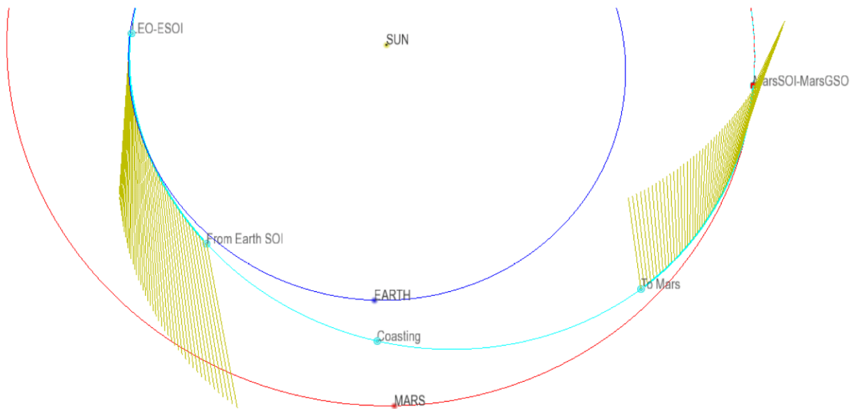
Figure 16: 2 MW SEP Mission to Mars
