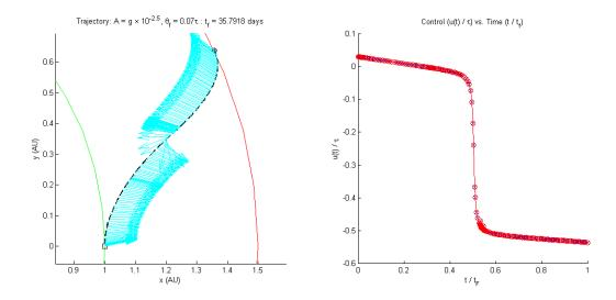
Figure 2.3: Plot of trajectory (left) and corresponding control (right) for acceleration magnitude  $A=10^{-2.5}g_0\gg \frac{\mu}{R^2}$  over the entire trajectory.
