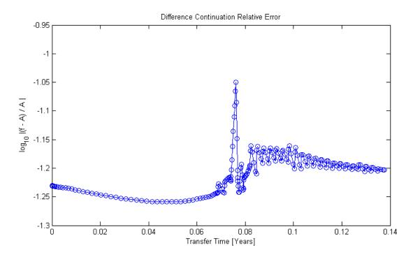
Figure 2.7: Plot of  $log_{10}(||\mathbf{f}^G| - A|/A)$ , a measure of the error incurred in the application of inverse dynamics on the trajectory produced by DC.
