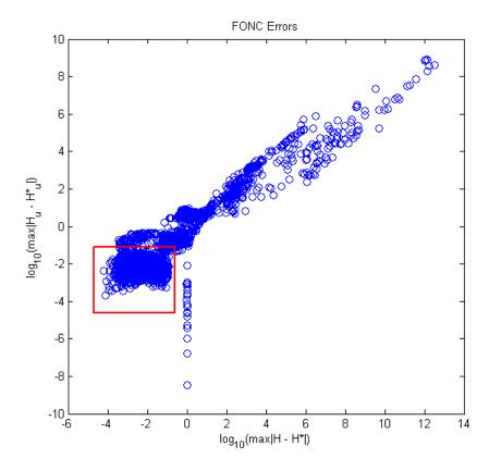
Figure 3.1: Plot of errors associated with meeting the FONC's. The red rectangle indicates the region of acceptable trajectories (error range:  $\mathcal{H} < 10^{-0.8}$  and  $\mathcal{H}_u < 10^{-1.2}$ ).
