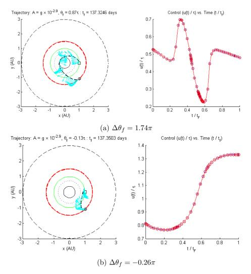
Figure 3.3: Branching point for trajectories at  $A = 10^{-2.9}g_0$ . Qualitatively different control behaviors are easily observed in this case.
