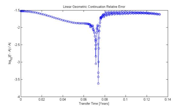
Figure 2.5: Plot of  $log_{10}(||\mathbf{f}^G| - A|/A)$ , a measure of the error incurred in the application of inverse dynamics on the trajectory produced by LGC.
