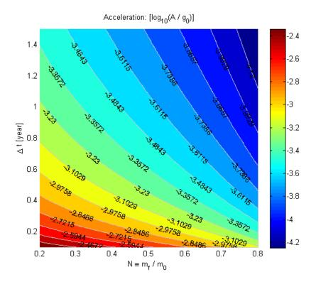
Figure 1.1: Minimum required acceleration magnitude (A) and maximum allowable transfer time ( $\Delta t$ ) as a function of desired payload fraction ( $\frac{m_f}{m_0} \in [0.2, 0.8]$ ) at a specified specific impulse ( $I_{sp} = 12000s$ ).
