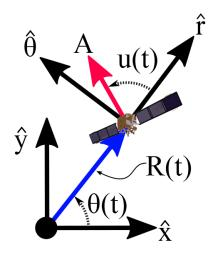
Figure 2.2: u(t) is the angle with respect to local coordinates of the acceleration vector
