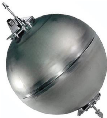
Fig. 16. Ariane 5 58 L hydrazine bladder tank ArianeGroup [24].
