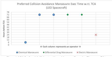
Figure 4: LEO Preferred Collision Avoidance Maneuver Execution Time w.r.t. TCA
