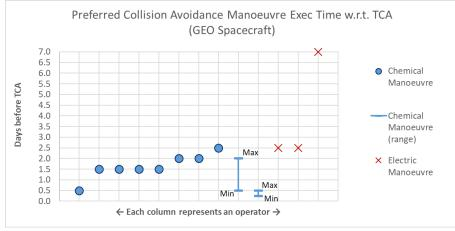
Figure 3: GEO Preferred Collision Avoidance Maneuver Execution Time w.r.t. TCA
