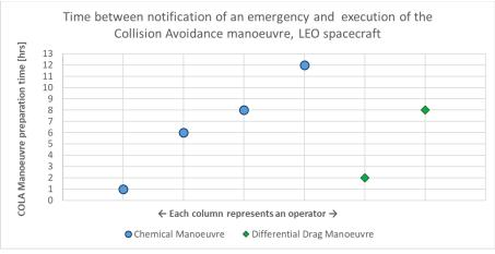
Figure 6: LEO Reaction Time
