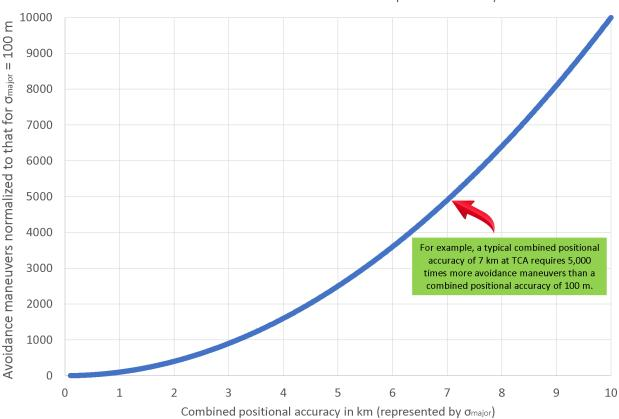
Avoidance maneuvers required versus combined positional accuracy, ratioed to avoidance maneuvers needed for a 100m combined positional accuracy
