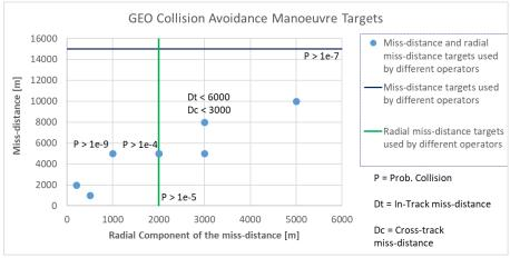
Figure 7: GEO Collision Avoidance Maneuver Targets
