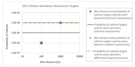
Figure 8: LEO Collision Avoidance Maneuver Targets
