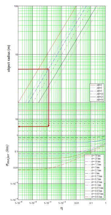
Figure 16. Nomogram to determine  $\sigma_{major}$  from r, d, and AR.
