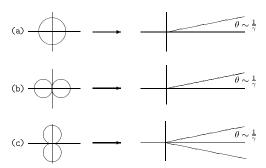
Radiation from an accelerated relativistic particle can be greatly enhanced. Part of this effect is due to the aberration of angles and part due to the Doppler effect.
